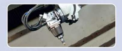
6-Axis Laserdyne 795XL Fibre Laser with Weld Capability
